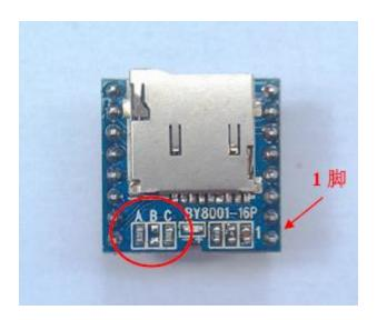
In the table below, '0' means grounding through a 3.3Kohm resistor, while '1' means open circuit. The module factory default setting is 010, but may be modified to suit customer's application. For serial control by MCU, recommended mode setting is '111'.
