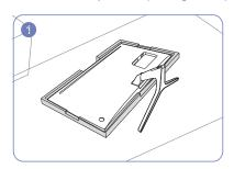
Place the protective Styrofoam (cushion) included in the package on the floor and place the product facing down on the Styrofoam, as shown in the image.
