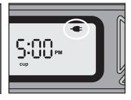
adapter is used to operate the feeder, the batteries function as a back-up power source in case of a power loss. When power adapter is being used as power source, the power adapter icon will appear at the top of the LCD screen.
