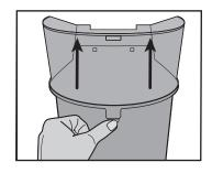
To Remove Conveyor: Pull back red conveyor latch to unlock. Lift to remove.
