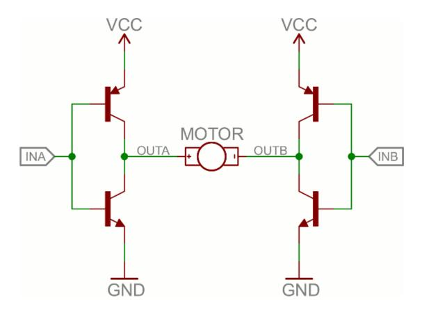
(Note: there's usually quite a bit more to a well-designed H-bridge including flyback diodes, base resistors and Schmidt triggers.)
