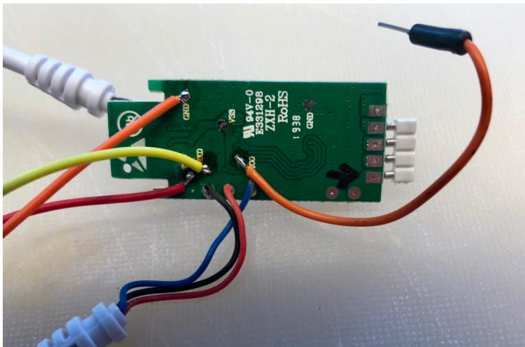
From the Arduino IDE, set your board as follows. This is an ESP8265 board.
