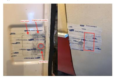
We could fiberglass the hole or add a plate to the front. Since the boler has yet to be painted, I am leaning towards fiberglass.
