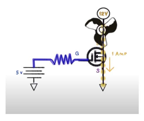
When voltage is applied between Gate and Source, current is allowed to flow between DRAIN and SOURCE.
