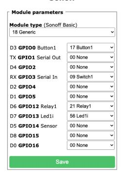
Connect Door sensor to GPIO3(TX on Sonoff S20 board) and GND.
