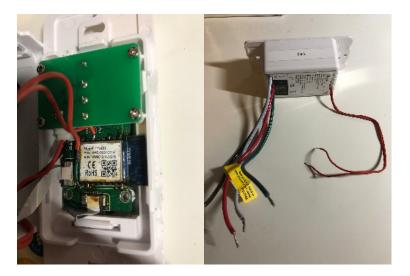
Wires were soldered onto GPIO-12 and GND and run through the back of the box.
