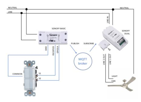
I used two sonoff devices because of the limited space. This setup allows you to use the switches as you normally would and also control the switch with your home automation.
