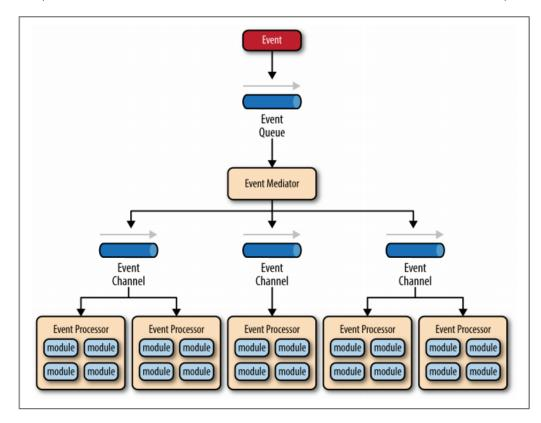
The pattern does not specify the implementation of the event queue component; it can be a message queue, a web service endpoint, or any combination thereof
