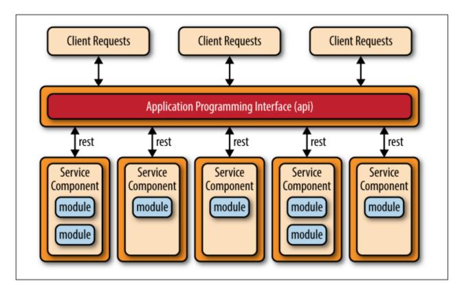
The API REST-based topology is useful for websites that expose small, self-contained individual services through some sort of API (application programming interface).
