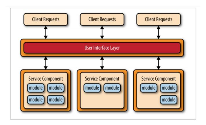
Service components contain one or more modules (e.g., Java classes) that represent either 27 a single-purpose function (e.g., providing the weather for a specific city or town) or an independent portion of a large business application (e.g., stock trade placement or determining auto-insurance rates). Desi gning the right level of service component granularity is one of the biggest challenges within a microservices architecture.
