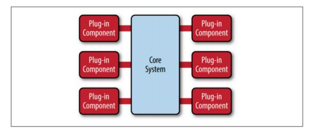
The core system needs to know about which plug-in modules are available and how to get to them. One common way of implementing this is through some sort of plug-in registry. This registry contains information about each plug-in module, including things like its name, data contract, and remote access protocol details (depending on how the plug-in is connected to the core system).
