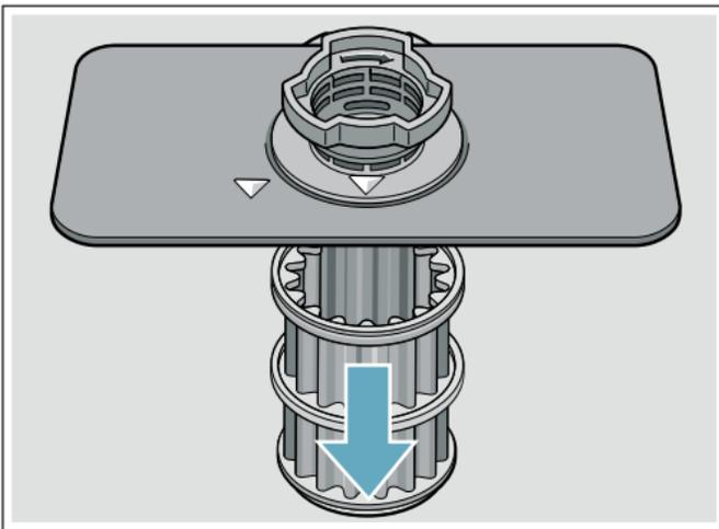
3. Rinse the filters under running water and use a soft brush to clean. Note: do not use abrasive brushes or steel wool, etc., as they may damage the filter.
