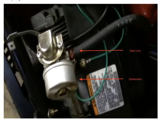
To remove the gas from the snow blower remove the clip and slide the gas line off. This will allow you to remove all of the gas from the system.
