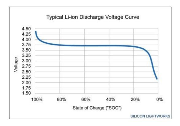
For a 3S battery, 80% of to capacity should have a voltage of it's nominal voltage (3.7v/cell) equal to 11.1v.
