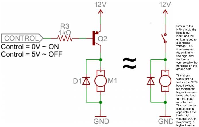
control input's high voltage. For example, this circuit wouldn't work if you were trying to use a 5V-operating Arduino to switch on a 12V motor. In that case it'd be impossible to turn the switch off because VB would always be less than VE.
