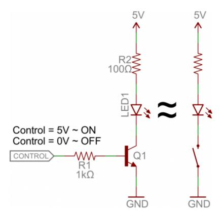
Our control input flows into the base, the output is tied to the collector, and the emitter is kept at a fixed voltage.
