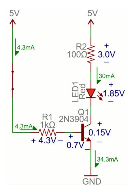
The resistor needs to be large enough to effectively *limit* the current, but small enough to feed the base *enough* current. 1mA to 10mA will usually be enough, but check your transistor's datasheet to make sure.
