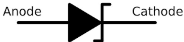
Taking advantage of their breakdown property, Zener diodes are often used to create a known reference voltage at exactly their Zener voltage. They can be used as a voltage regulator for small loads, but they're not really made to regulate voltage to circuits that will pull significant amounts of current.
